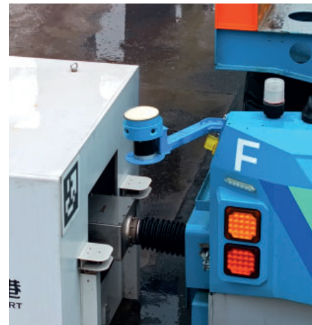
The QCC charging connector and the ART in mated state for charging.
