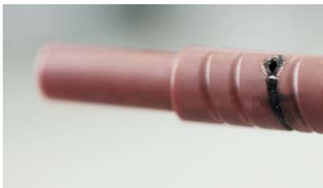
Breakdown with non-compliant plug-in connector
