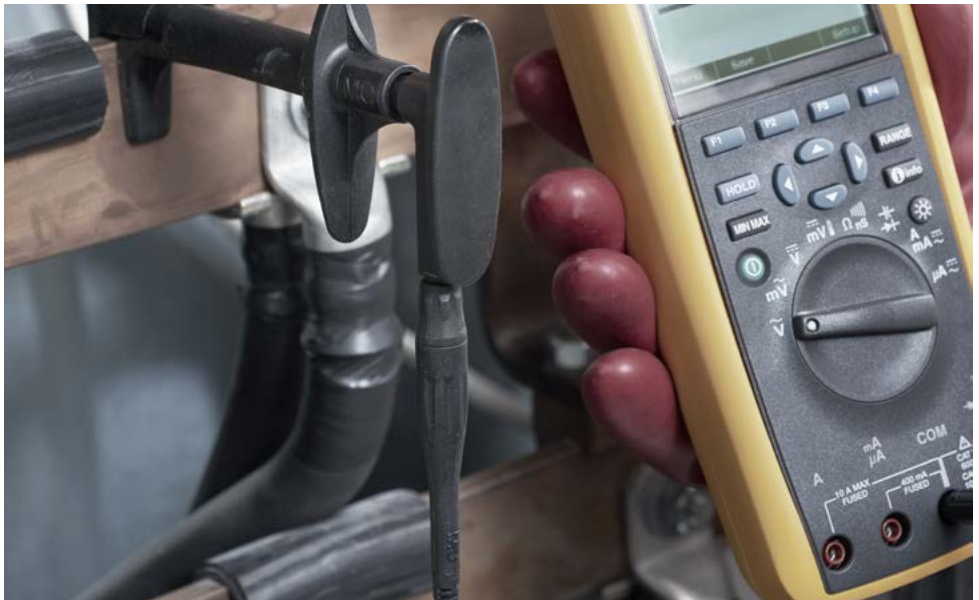
House junction box and examples of test accessories for CAT IV.
